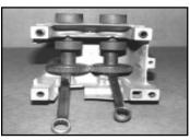
The shafts must be supported with a .165" - .185" spacer placed between the housing and the gear during assembly.
