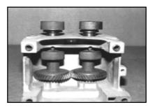
With the weights positioned on top, install the gears with the helix angled to the outside on the bottom of both gears. Time the balance shafts by lining up all of the weights centered and facing toward you.
