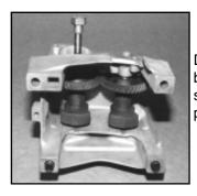
Disassemble the balancer by pressing the shafts apart from the oil pump side.
