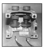
The spacers are made from 11/16" open end wrenches. Press the shafts back together with these spacers in place to get them properly positioned.
