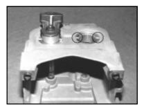
Be sure to install the new bearing even with the bottom of the chamfer in the housing so the oil will feed out to thrust faces through the slots machined in the housing.
