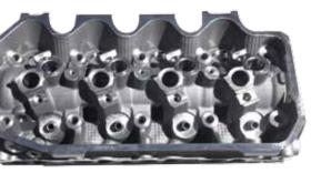
This cylinder head boasts thicker (.4375) decks to provide improved heat transfer along with a better platform for decking. CNC machined guides and seats increase flow. For greater thermal conductivity, EQ has redesigned the water flow.
