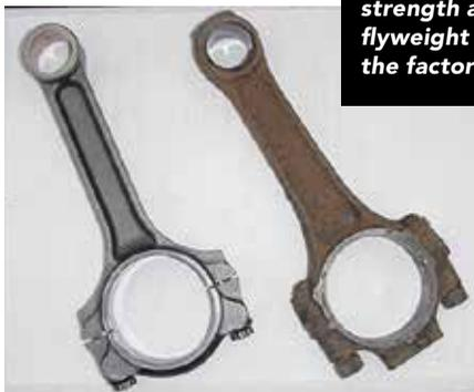
**The Scat Industries I-beam connecting rods added significantly to our diet plan, while adding strength and durability. Our new rods came in at a flyweight 574 grams. A full 179 grams lighter than the factory rods.**
