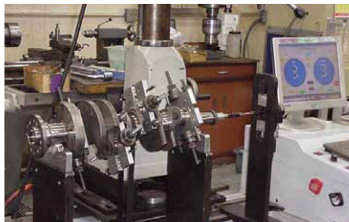
**Our bobweight was significantly lower than the Scat target weight. After we almost launched our crank out of the CWT balancer, a portion of the crank counterweights were removed on the crank grinder.**
