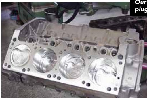
**Our assembled shortblock, still missing freeze plugs at this point.**
