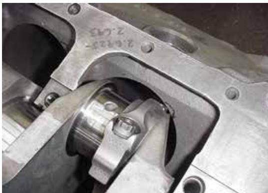
**When a few of the bearings were installed the crank was laid and a rod and piston were installed to check for clearance. There is very little that needed to be removed from the bottom of the cylinders to clear the connecting rods. There is plenty of clearance around the cam, the pan rails and the bottom of the cylinders for our 4.000" stroke crank.**
